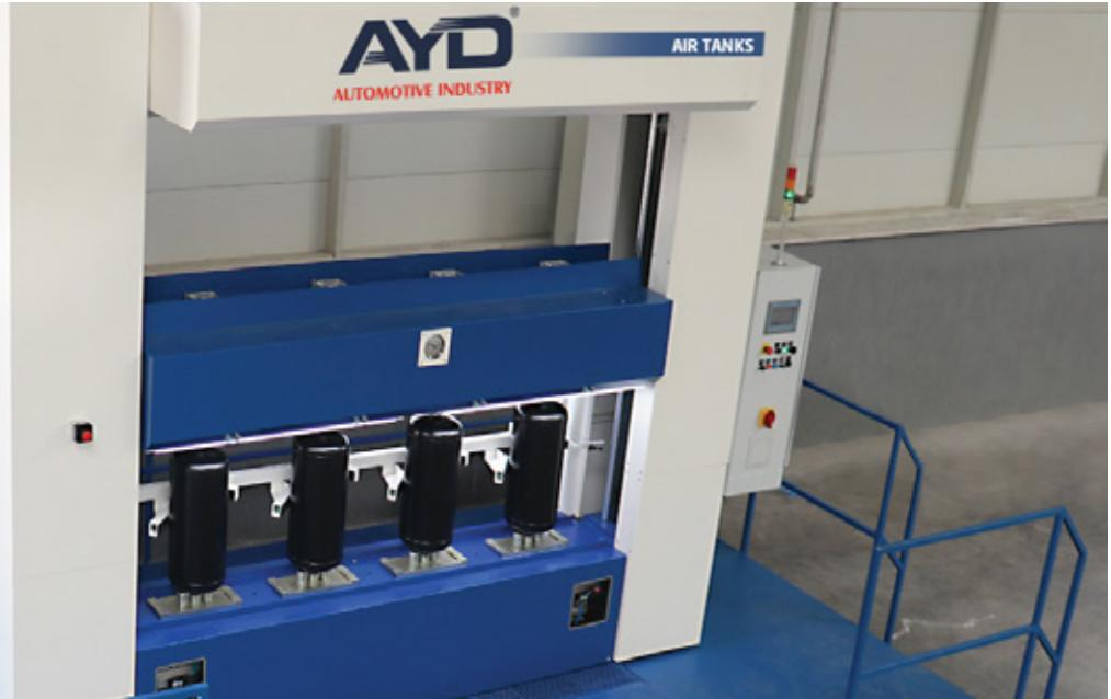
We are doing 100% high pressure tests to all our products as specified in the CE directives. We always prioritize product and vehicle safety and test the sealing and compressive strength of the each products cylinder, cover and sleeve surfaces under the test conditions which are 1.5 times higher then the maximum working pressure ( $P_s = P_{max} \times 1.5$ ).
